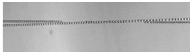
FIGURE 8 X-coupler written with crossing pearl-chain waveguides
