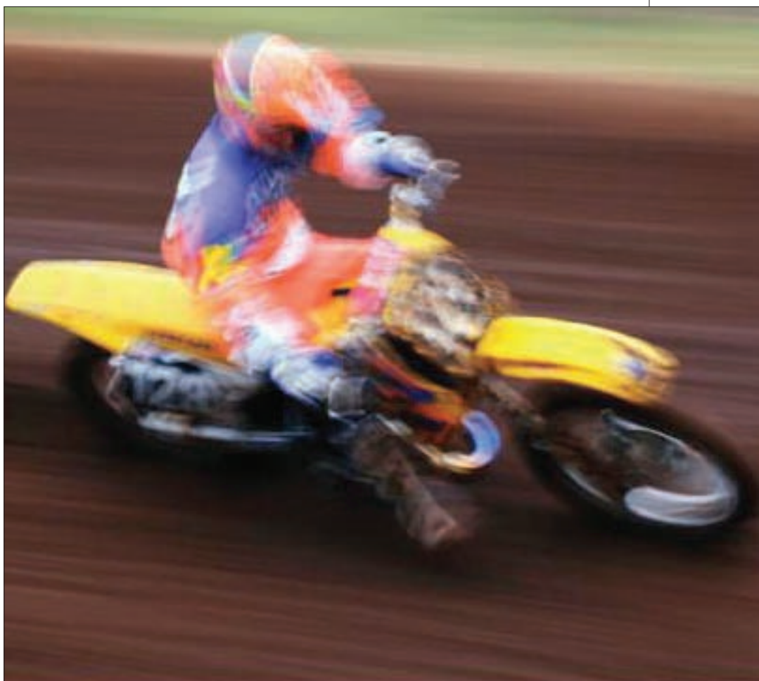
Figure 2. Motorcyclist in motion. The image is blurred because the object noticeably changes position during exposure. From position change \Delta x (which can be assessed from the blurring) and speed v of the motorcyclist, the camera exposure time can be readily determined: \tau_{\text{exp}} = \Delta x/v (if the camera is assumed to be stationary for the sake of simplicity). This same concept forms the basis for evaluation of the subfemtosecond x-ray pulse duration from the x-ray photoelectron spectra shown in Fig. 6.
