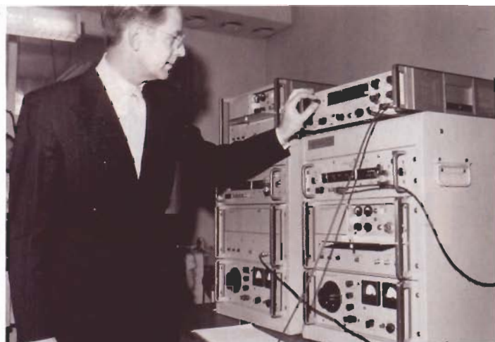
A laboratory engineer compares time measured by his atomic clock with the time shown on clocks that have just flown around the world
