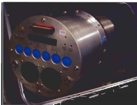
High flyer – it may not be on everyone's packing list, but the tissue-equivalent proportional counter is an important device for measuring the exposure to cosmic radiation when flying.
