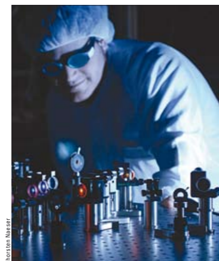
The laboratory for attosecond physics at Garching produces chirped multilayer mirrors for its research. Volodymyr Pervak (left) and Adrian Cavalieri (bottom middle) are seen examining the mirrors. An array of multilayer mirrors (top middle) compresses ultrabroadband laser pulses to 1.5 wave cycles. The attosecond X-ray pulses produced with them allow the control and real-time observation of atomic-scale electron motion. Lund's attosecond stroboscope is shown far right.
