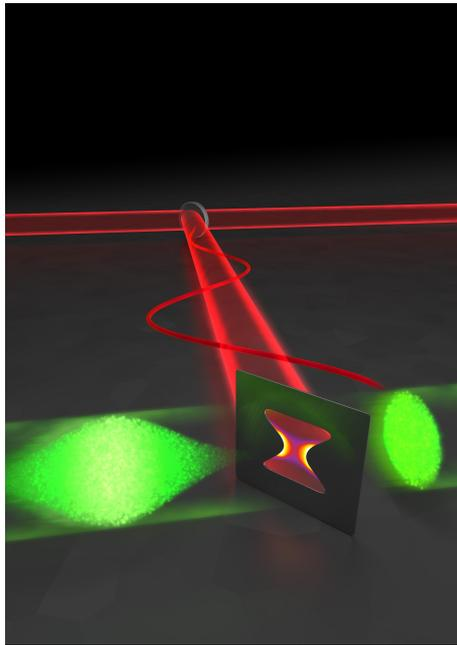
*Image description: Pulses from electrons (green, coming from the left) meet a micro-structured antenna which runs on laser-driven terahertz radiation (red). Thus the duration of the electron pulses shorten to few femtoseconds. The shorter the duration of the electron pulses, the better the films of atoms inside of solids or molecules.*
