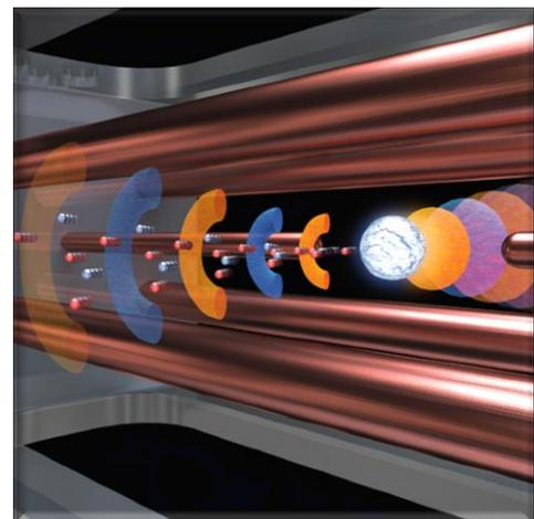
Blasting a bunch of protons from such a plastic microsphere requires extremely powerful and efficient laser systems. The PHELIX laser in Darmstadt, which was used in the experiments, has the necessary specifications. It is capable of producing laser pulses that last for 500 femtoseconds (1 femtosecond is equivalent to a millionth of a billionth of a common second), and transport
