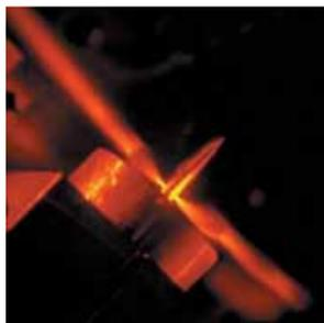
*A high-intensity few-cycle (7-fs) red light beam pumps the neon-gas attosecond-pulse source. The characteristic fluorescence emission from neon originates from the ionizing atomic gas as it streams out of the volume inside a thin metal tube with a couple of holes in its wall to transmit the pump laser and the emerging x-ray beam. (Photo courtesy of G. Tempea; Vienna U. of Technology)*
