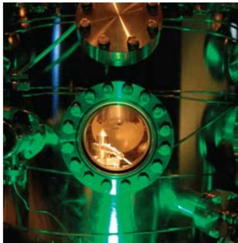
The attosecond-scale measurement scheme uses a commercial Ti:sapphire laser to deliver waveform-controlled few-cycle, 5 fs near-infrared (750 nm) laser pulses at a repetition rate of 4 kHz. The laser pulses produce isolated coincident 300-attosecond EUV pulses used for real-time observation of rapid electron motion inside atoms, molecules, and solids. (Courtesy of Max-Planck-Institut für Quantenoptik/Thorsten Naeser)
