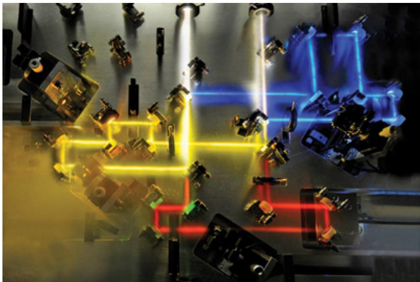
A photonic system produces custom-shaped sub-femtosecond light transients used to probe the behavior of electrons within atoms. To create the transients, a supercontinuum is first divided into three channels (seen as blue, yellow, and red); beam parameters for each channel are manipulated before recombining the light (white). (*Courtesy of E. Goulielmakis*)
