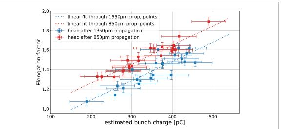
**Figure 7.** Elongation of the first cavity versus estimated initial bunch charge using the charge–energy correlation in the beam loading regime, for two different positions within the PWFA stage. Plasma density was at  $4 \times 10^{18}$  cm<sup>-3</sup> in both cases. The dotted lines represent a linear fit through each data set, just to guide the eye.
