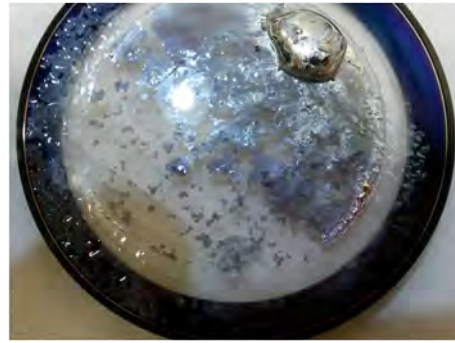
b) Cracking of HR coating under O-Ring pressure
